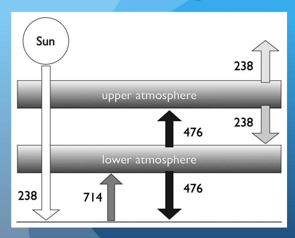
$$T_{two\_layers} = 4\sqrt{\frac{714}{5.67 \cdot 10^{-8}}} = 335K = 62^{\circ}C$$
