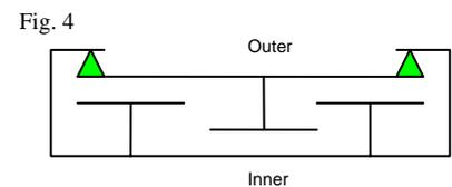
The '120 patent also has dependent claim 2: “Modules as defined in claim 1 wherein the steel baffles are oriented with the panel sections disposed at angles for deflecting projectiles such as bullets able to penetrate the steel plates.”
