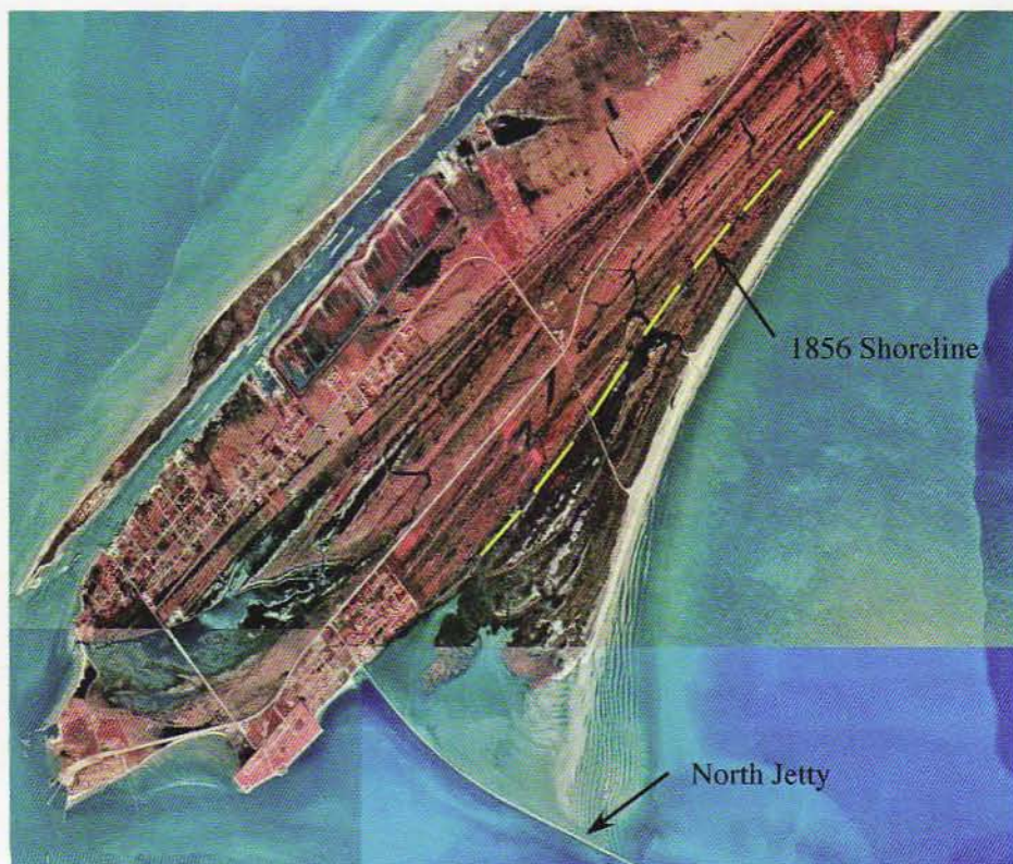
Figure 1.4. Along Bolivar Peninsula, the longshore drift system delivers sand toward Bolivar Roads, the pass between Galveston Island and the peninsula. But before the sand reaches the inlet it is blocked by the North Jetty. If you drive to the area just east of the jetty, you can see the extensive beach that has formed from sand trapped on the "up-drift" side of the jetty. Note the location of the 1856 shoreline (dashed line) before the jetty was constructed. Note also the linear features that extend along the peninsula. These beach ridges, separated by depressions or swells, formed when the peninsula was growing naturally. Photo from the U.S. Geological Survey.
